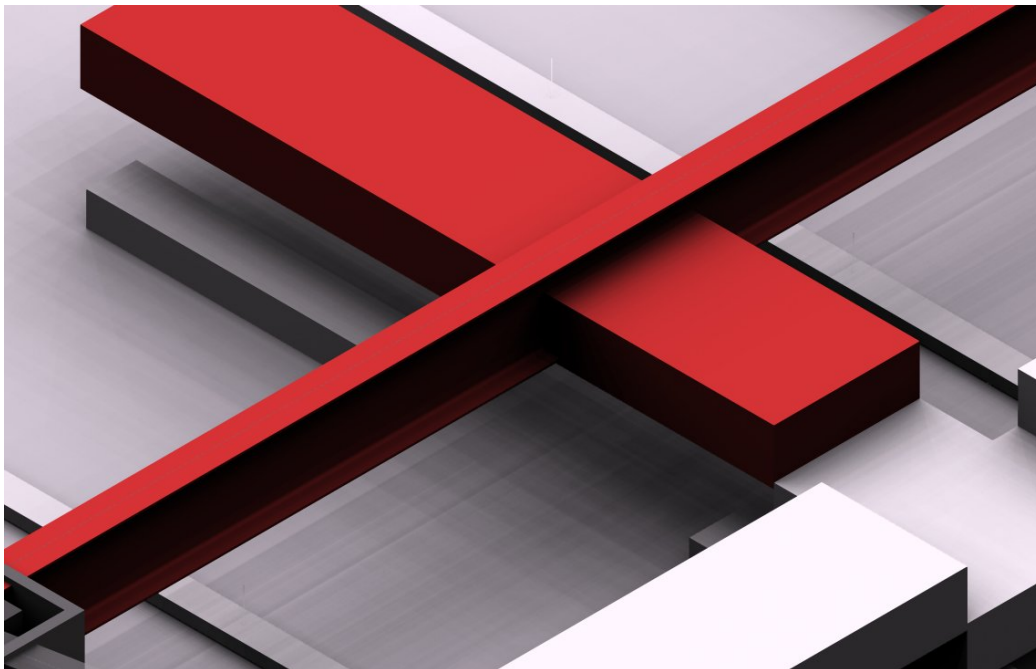
Figure 1: Beam and duct clash in core corridor
